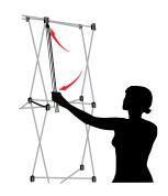
Insert magnetic bars into frame. Start at the top, push the pointed end into the slot. Slide bottom of bar over metal peg to lock into place. Insert next bar into bottom of previous bar.
