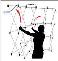
Open the frame to its full open position. Once the frame is completely expanded, it will remain in the fully opened position.
