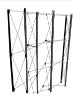
Continue inserting magnetic bars on front and then insert one column of bars on each back corner.
