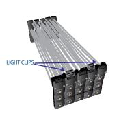
Remove frame from the case and place on table top with the light clips on top and facing towards you.
