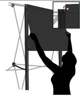
Attach fabric panels. Locate notches on top of panel and slide notch over peg cap. Unroll panel allowing it to attach magnetically to half of the magnetic bar as it unrolls. Repeat for all front panels.
