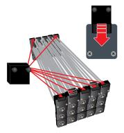
Insert plastic peg caps into slots on upper part of frame. Four on the front and two on the back.
