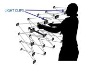
Open the popup frame halfway by pulling up and out on the center of the frame.
