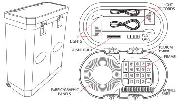
To store the unit, remove panels, endcaps, channel bars, peg caps and lights. Collapse frame. Stack panels and graphics with fabric and graphics side up. Roll up and insert into case. Insert frame and channel bars into case. Pack lights and peg caps into case cover. Close lid and secure all latches.
