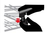
Once the frame is open halfway, slide the halogen lights onto the light clips and insert the power cord into the back of the light.
